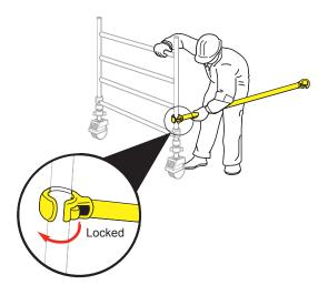
Position the second end frame as shown and fit the other end of the horizontal brace on to the vertical, just above the bottom rung. Fit a second horizontal brace between the bottom rungs on the other side of the frames to square the tower.
